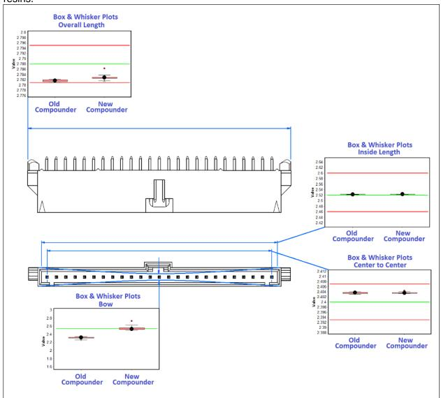
4.4 Conducted trial assembly runs with housings run with resin from both compounders
